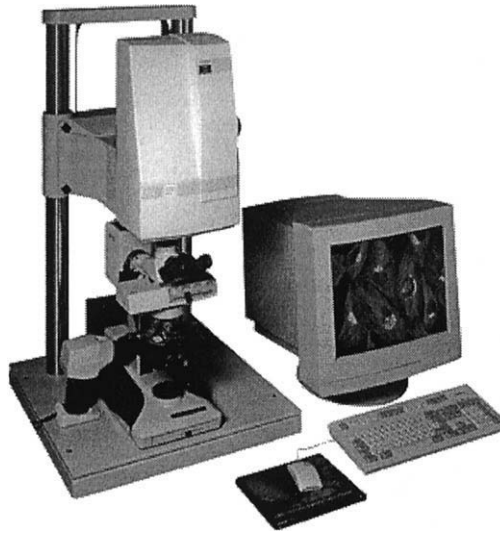
Fig. 17 The Bio-Rad MRC-1024 confocal laser scanning microscope which is a single point-scanning system. (Courtesy of Bio-Rad Microscopy Division, Hemel Hempstead, UK.)
