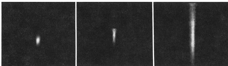
Fig. 4 Projections from the side of 0.5\text{-}\mu\text{m} beads at different distances from the coverslip. The beads are in water and were scanned with a \times 40 NA 0.95 lens. Left: 5\ \mu\text{m} from coverslip. Middle: 30\ \mu\text{m} from coverslip. Right: 115\ \mu\text{m} from coverslip.
